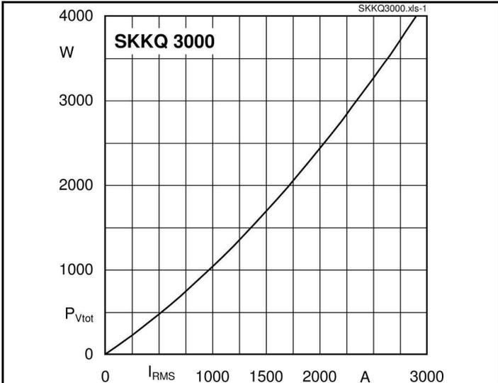
Fig. 1 Power dissipation per module vs. rms current
