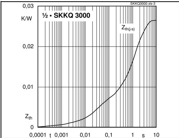
Fig. 3 Transient thermal impedance  $Z_{th(j-s)}$  vs. time
