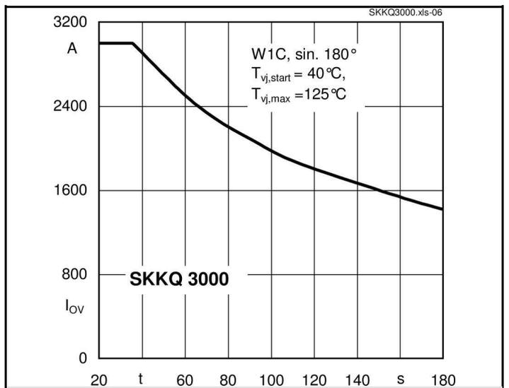
Fig. 6 Typ. overload current vs. time (natural cooling)
