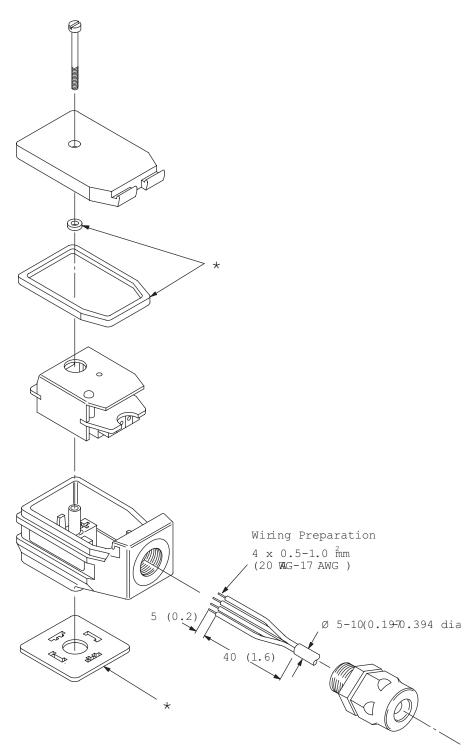
\*All seals must be fitted correctly at plug installation to provide protection to IP67 (IEC 529).
