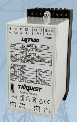
LQT400 is a configurable multi transducer for all electrical networks. Any two measurable electrical quantities can be linked to the two analog outputs.
