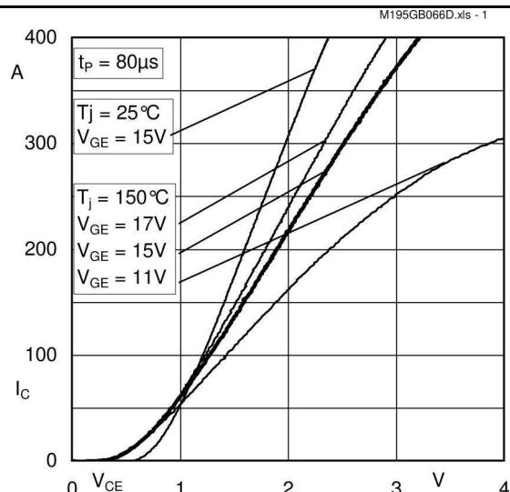
Fig. 1 Typ. output characteristic, inclusive  $R_{CC} + EE$
