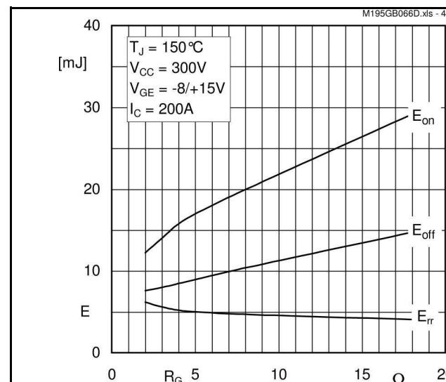
Fig. 4 Typ. turn-on /-off energy =  $f(R_G)$
