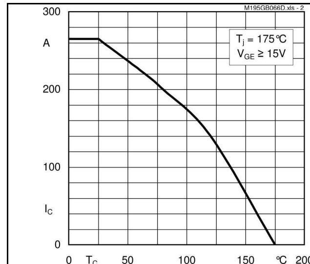
Fig. 2 Rated current vs. temperature  $I_C = f(T_C)$
