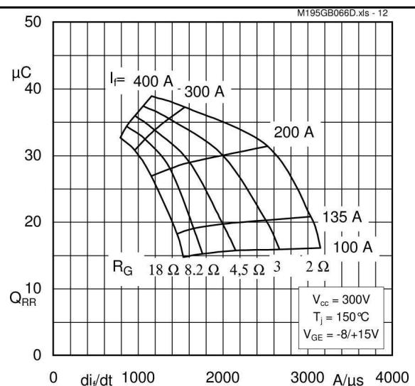
Fig. 12 Typ. CAL diode recovered charge
