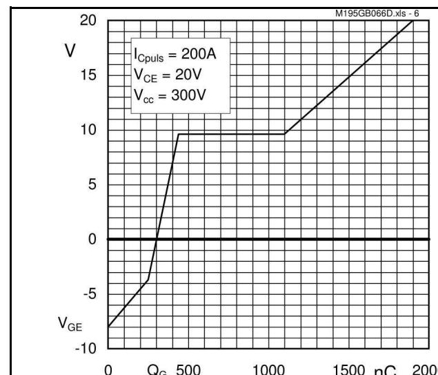
Fig. 6 Typ. gate charge characteristic
