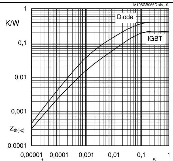
Fig. 9 Transient thermal impedance of IGBT and Diode
