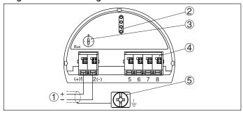
Fig. 30: Electronics and terminal compartment, single chamber housing
