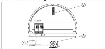
Fig. 27: Terminal compartment, double chamber housing
