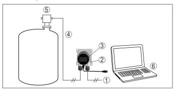
Fig. 40: Connection of VEGADIS 82 to the sensor, adjustment via PC with PACT-ware
