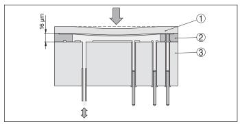
Fig. 2: Configuration of the CERTEC® measuring cell in VEGABAR 82
