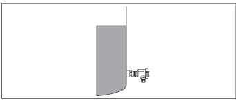
Fig. 24: Level measurement in a vessel with VEGABAR
