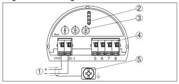
Fig. 28: Electronics and terminal compartment, single chamber housing
