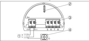
Fig. 31: Terminal compartment, double chamber housing
