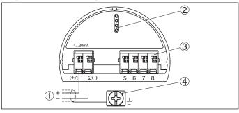
Fig. 25: Electronics and terminal compartment, single chamber housing
