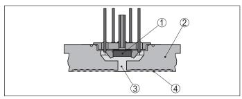
Fig. 3: Configuration of the piezoresistive measuring cell in VEGABAR 83
