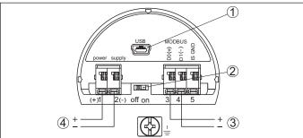
Fig. 32: Terminal compartment
