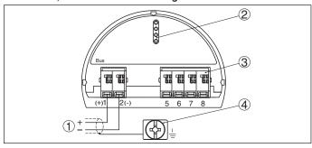
Fig. 29: Terminal compartment, double chamber housing
