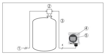
Fig. 38: Connection of VEGADIS 81 to the sensor
