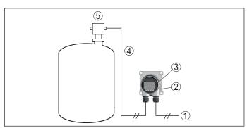
Fig. 39: Connection of VEGADIS 82 to the sensor
