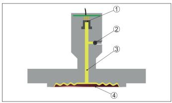
Fig. 1: Configuration of a chemical seal system
