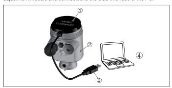
Fig. 35: Connection of the PC via VEGACONNECT and USB
