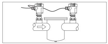
Fig. 13: Electronic differential pressure measurement through Master/Slave combination
