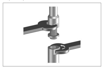
Fig. 21: Exchanging the cable or rod
