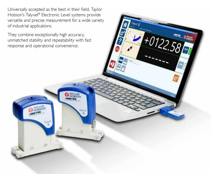
Incorporating a compact, highly stable, pendulum transducer in the Level Unit and interfacing directly to a tablet PC or laptop with dedicated software, Talyvel® 6 provides rapid and simple reading of angle of tilt and measurement relative to gravity. It is simple to calibrate and operate, with a fast measurement response time.
