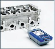
Robust and portable surface roughness testers
