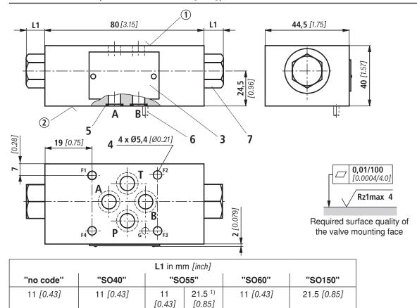
1) Maximum dimension on the side of the check valve use
