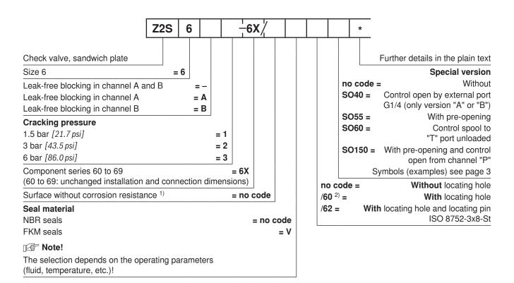
Corrosion-resistant surface upon request: e.g. "J50" thick layer passivated (DIN 50979 Fe//Zn8//Cn//T0)
