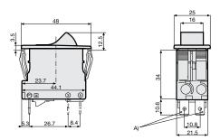
A) Quick connect terminal, IEC 61210, A6.3-0.8 mm
