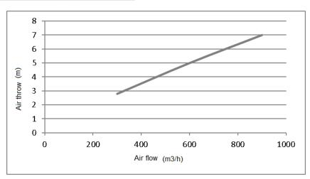
CAUTION! The difference in temperature between the delivery air and the ambient air can significantly influence the air throw.
