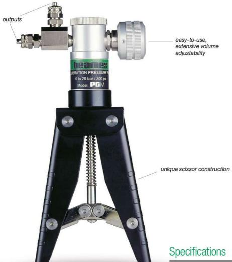
The PGM is a hand-operated pressure calibration pump that uses air as its pressure medium. The extremely accurate volume control provides the excellent fine adjustment of pressure. The pump's unique and sturdy construction makes the PGM the ultimate field calibration pump.
