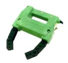
Solid-state controls allow the operator to use AC magnetic fields for surface indications or DC magnetic fields for sub-surface indications, to meet all inspection needs.
