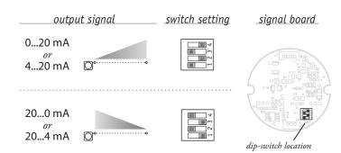
The output signal direction can be reversed at any time by simply changing the dip-switch settings found on the internal signal board. After the settings have been changed, adjustment of the Zero and Span trimpots will be required to precisely match signal values to the beginning and end points of the stroke. To gain access to the signal board, remove four Allen-Head Screws and remove end cover bracket.
