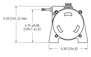
\* tolerance = +.005 -.001 [+.13 -.03] \*\* tolerance = +.005 -.005 [+.13 -.13]
