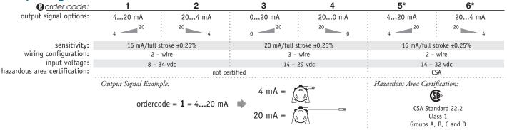
\*IMPORTANT: intrinsically safe when powered from a CSA certified zener barrier rated 28 VDC max, 110 mA max per installation drawing#677984
