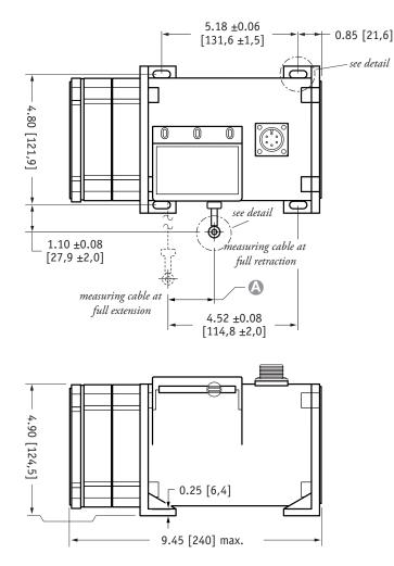
DIMENSIONS ARE IN INCHES [MM] tolerances are 0.03 IN. [0.5 MM] unless otherwise noted.
