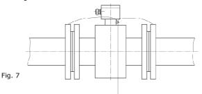
When using pipes lined with electrical insulation, plastic tubing or concrete conduits, a separate earthing washer is used to earth the measuring media. The earthing washer is installed between the pipeline connection and the sensor's flange and the ring's inside contacts the media. Contrary to the diagram shown below, one earthing washer on the inflow side is sufficient. However, if bidirectional measurements are to be taken, one earthing washer must be installed on either side.
