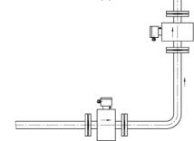
Fig. 2 Installation in horizontal and vertical pipeline
