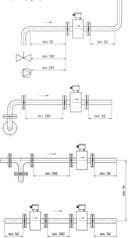
Fig. 5 Installation between tees, valves and pumps
