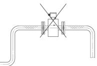
Fig. 6 Installation at highest point
