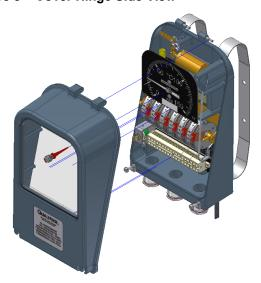
Figure 9 - Front Cover Removal
