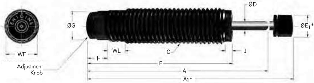
\*Note: A<sub>1</sub> and E<sub>1</sub> apply to button models. One Hex Jam Nut included with every shock absorber.
