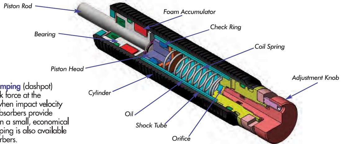
**Constant orifice area damping** (dashpot) provides the largest shock force at the beginning of the stroke when impact velocity is highest. These shock absorbers provide high-energy absorption in a small, economical design. This type of damping is also available in adjustable shock absorbers.
