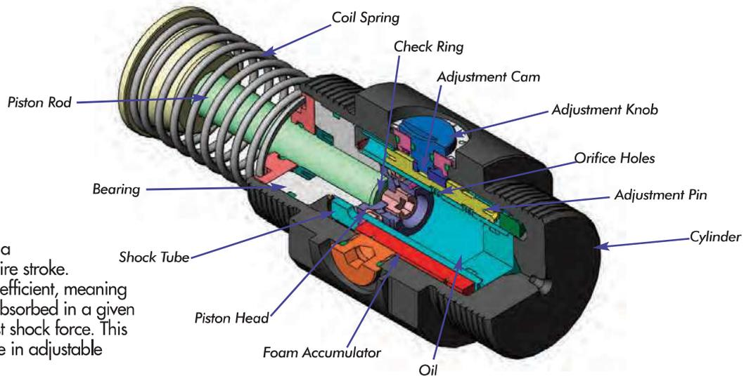
**Conventional damping** allows linear deceleration by providing a constant shock force over the entire stroke. This standard design is the most efficient, meaning it allows the most energy to be absorbed in a given stroke, while providing the lowest shock force. This type of damping is also available in adjustable shock absorbers.
