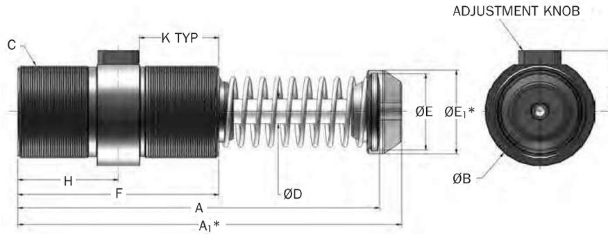
\*Note: A<sub>1</sub> and E<sub>1</sub> apply to urethane striker cap accessory.
