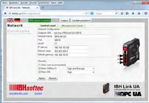
The IBH Link UA is an OPC UA Server/Client module with integrated firewall for the SIMATIC S5, S7-200, S7-300, S7-400, S7-1200, S7-1500 and LOGO! (Ethernet versions) PLC. It is a compact unit for DIN rail mount with four Ethernet ports and a 24V power supply.
