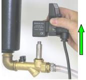
2.Press the TEST button to empty the unit of any residual condensate and to depressurise the FLUIDRAIN COMBO valve.
