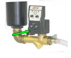
9. Place the connector gasket on the connector, plug the connector on the timer as illustrated below and tighten the screw (max. torque 1Nm). Make sure both gaskets are secured properly to ensure IP65 rating.
