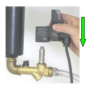
12. Press the test button to check the valve function.
