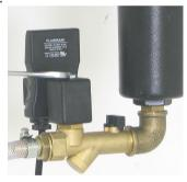
6. Unscrew the valve shaft using a 23 mm wrench.
