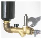
Do not use the valve shaft as a lever!
