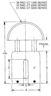
Tensioner body and chain guide width dimensions are same for both standard and compact series, only closed height K/L and guide radii differ.
