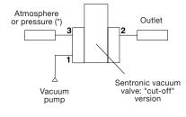
\*To accelerate vacuum control, it is possible to apply pressure (max. 2 bar) instead of atmospheric pressure to port 1 in the V1 Shut-off version or to port 3 in the V3 Shut-off version
