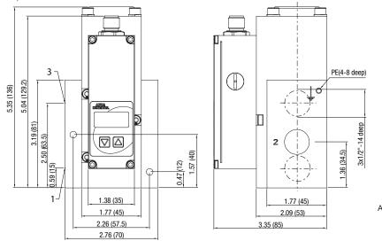
A) Thread M5 - depth 10 (on opposite side); tapped through-hole for M4 screw.
