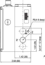
A) Thread M5 - depth 10 (on opposite side); tapped through-hole for M4 screw.
