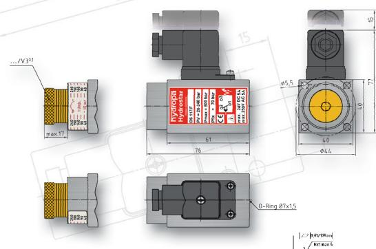
$^{1)} {\sf The}$  scale is only provided for orientation. The exact configuration of the switching pressure should be realised with a pressure gauge.
