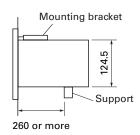
\* 70% or more of the analyzer weight should be supported at the bottom of the case. (In case of mounting panel or 19-inch rack provide a support at the end of casing.)
