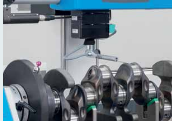
The probe is swiveled by 90° for roughness measurements on pin bearings.
