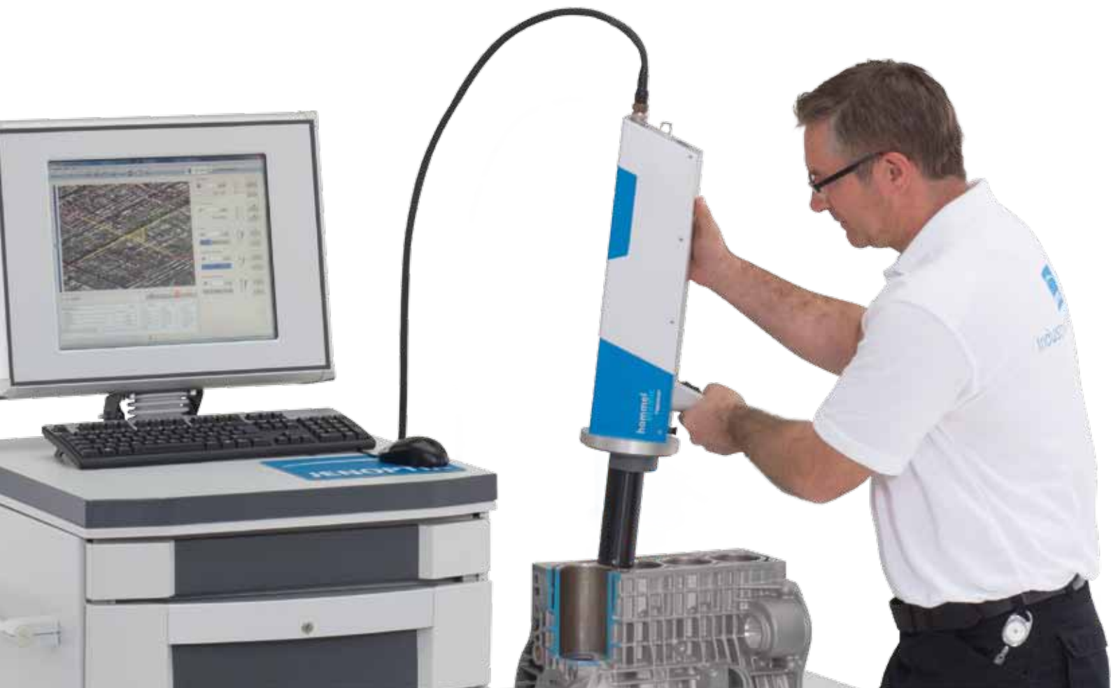
HOMMEL-ETAMIC toposcan OR150 with mobile workstation
