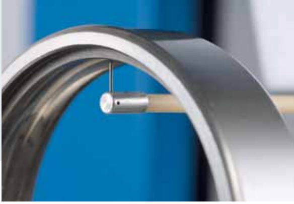
Combined roughness and contour measurement
