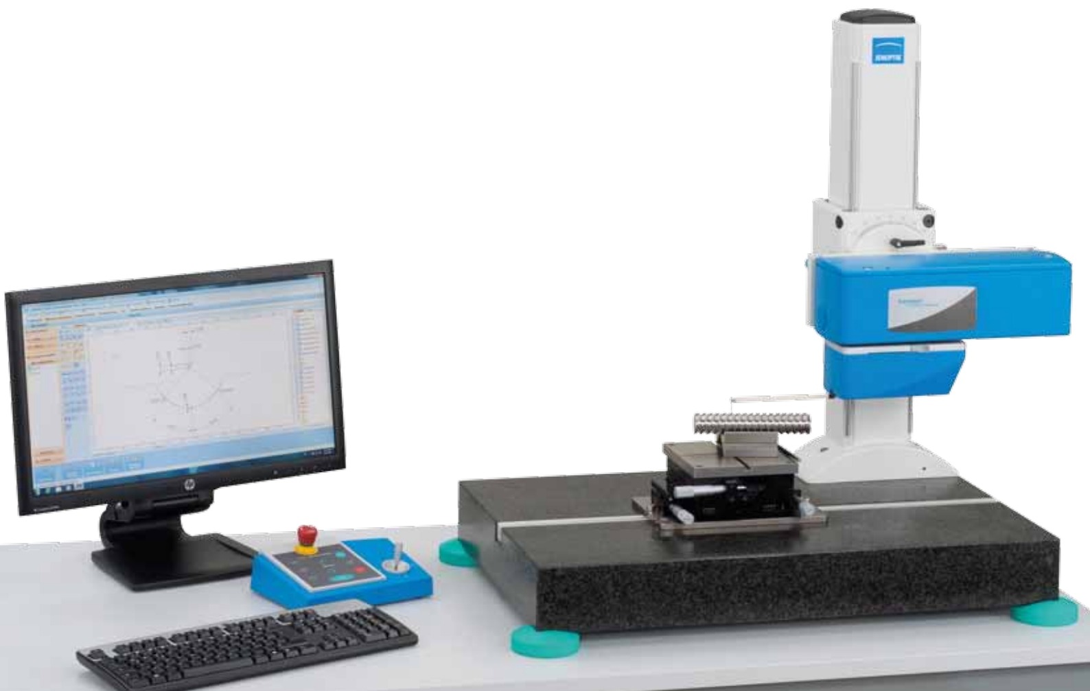
HOMMEL-ETAMIC surfscan with optional vee-block
