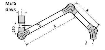
MET for ceiling mounting, excluding ceiling bracket MTI. MEV for wall mounting, including wall bracket MVK.
