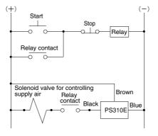
Remark: The above diagram shows the case when the solenoid valve for controlling supply air is normally open (NO; order code: -11).
