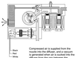
nozzle into the diffuser, and a vacuum is generated when air is sucked into the diffuser from the gap between the nozzle and the diffuser. The vacuum level rises until it exceeds the set vacuum level, causing the vacuum switch to activate.
