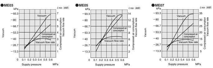
Remark: Graphs are for each single ejector unit. If the unit with solenoid valve requires the same vacuum level, set the supply pressure 0.03~0.05MPa [4.4~7.3psi.] higher than the single ejector unit's case. 1MPa = 145psi. 1kPa = 0.145psi. -100kPa = -29.54in.Hg 1 ℓ /min = 0.0353ft3/min.
