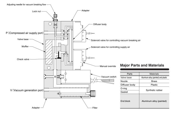
When energizing a solenoid valve for controlling supply air (generating vacuum)
