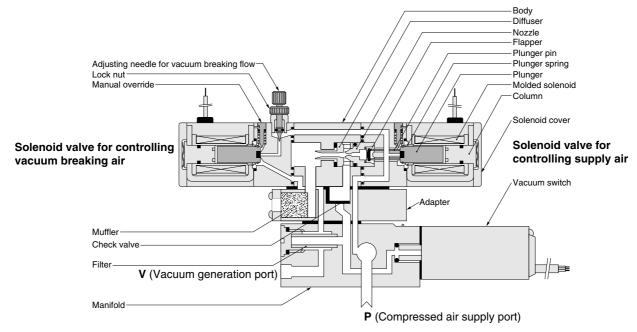
•When energizing a solenoid valve for controlling supply air (generating vacuum)
