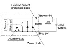
Brown: Lead wire for connecting the (+) polarity that activates the switch Black: Lead wire for connecting the load Blue: Lead wire for connecting the (-) polarity
