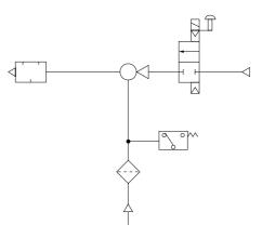
With twin solenoid valves and vacuum switch • GME05-E2-E
