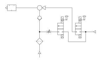
With single solenoid valve and vacuum switch • GME05-E1-E
