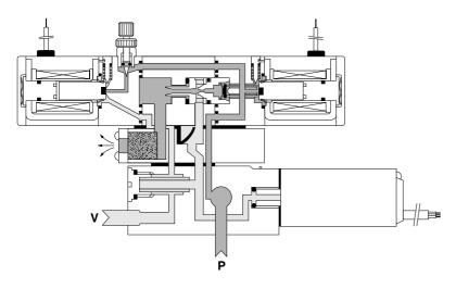
When energizing solenoid valve for controlling vacuum breaking air
