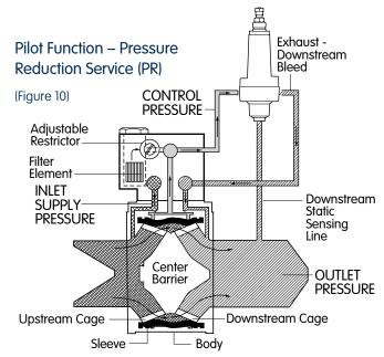
For pressure regulation, the pilot senses downstream pressure. A demand for flow will slightly reduce downstream pressure and will open the pilot valve. The effective opening of the pilot valve is regulated by changes in the downstream pressure sensed.
