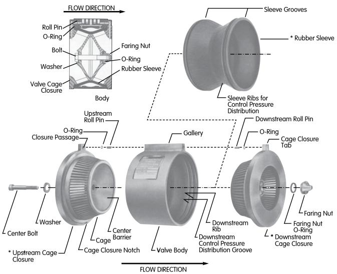
\* Cage closures are interchangeable. Rubber sleeve can be installed in either direction.
