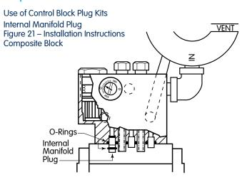
Downstream monitoring and passive upstream monitoring applications require the use of an internal inlet plug to block the pilot supply and to prevent pressure build-up in the intermediate pipiing between the two Axial Flow Valves. This plug is available as a retrofit kit; order Kit No. 74036K001. (Composite Block)
