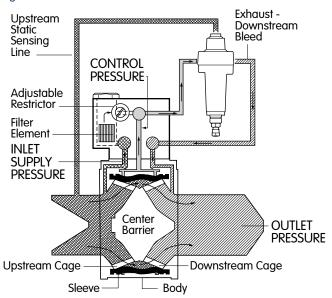
For back-pressure regulation and relief-valve operation, the pilot senses upstream pressure. An increase in upstream pressure above the dead-end shut-off† pressure causes the pilot valve to open and exhaust control pressure.
