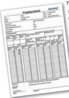
the tool to the computer and the test certificate indicating date and time is displayed as a pdf document. This is how you record the trouble-free function of the tool. User errors, such as premature stopping and retraction of the hydraulics or other faults that could prevent correct crimps are displayed. You can then print out the test report. Because the system uses the realtime clock of the connected computer, the test reports are recognised by QA systems.
