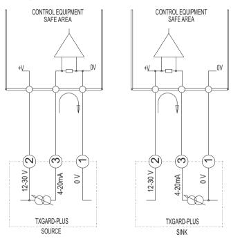
Diagram 3: Electrical connections to TXgard-Plus
