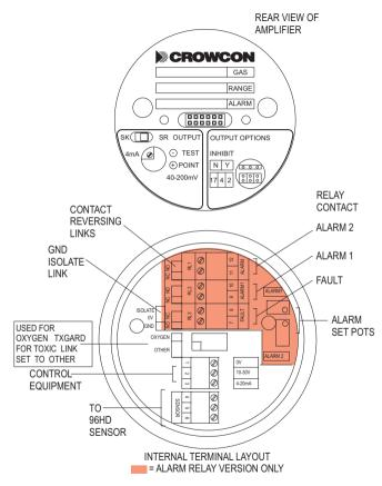
Diagram 2: Terminal and amplifier layouts
