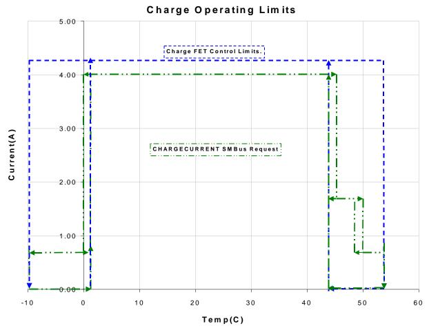
NOTE: If not charging & temperature > 45C then the battery enters Charge-Inhibit where ChargingCurrent() = 0 & ChargeVoltage() = 0 until temperature <= 44C
