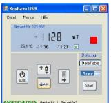
Connected Handheld Tesla / Gauss Meter KOSHAVA5 can be operated simultaneously on the device and the software
