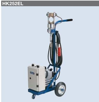
• with crimping head, 130 kN crimping force
