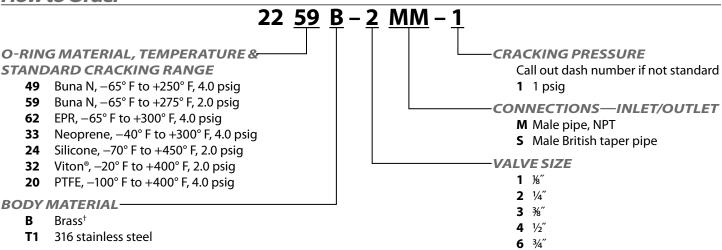
$\dagger$  For PED applications, brass bodies are limited to a maximum temperature of +100° F (+38° C).
