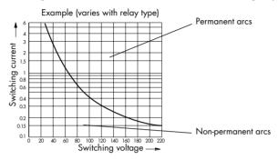
The area below the curve ensures a service life of  $\geq 1 \times 10^6$  operating cycles (90 % success of test samples).
