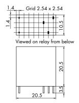
Hole diameter contacts 1.2 mm Hole diameter coil 1.0 mm
