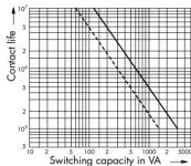
resistive load ---- inductive load,  $\cos \varphi = 0.4 \dots 0.7$
