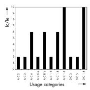
Ic = making-, breaking current le = rated operating current Ic/le = 1 for the usage categories not shown in the diagram
