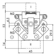
Auxiliary contact Blow-out magnet I Quick-action fastening
