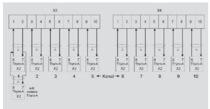
FIG. 12 CONNECTION DIAGRAM MAINS LOAD OPTIMIZATION WITH THYRO-POWER MANAGER
