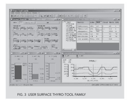
Power controllers of the Thyro-A series can be operated conveniently with the PC software Thyro-Tool Family and settings can be made. The prerequisite for working with the Thyro-Tool Family is that there is a connection between the PC and power controller. This means that measured values can be visualized and parameters displayed. If the Thyro-A is not operated in Thyro-Tool mode, certain parameters can be altered. In Thyro-Tool mode, almost all parameters can be altered.
