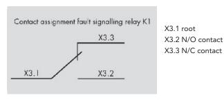
Fault signalling relay K1 has a changeover contact. Messages that cause the fault signalling relay to switch can be set with Thyro-Tool Family. In the default state, fault signalling relay K1 functions on the closed circuit principle.
