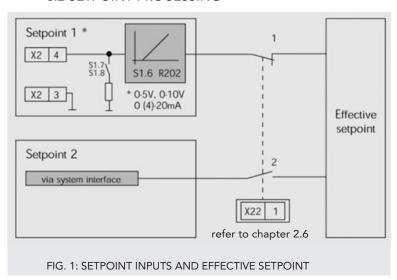
The user can adapt the setpoint signal to process controllers or to the automation system (see page 42, Set point input range).
