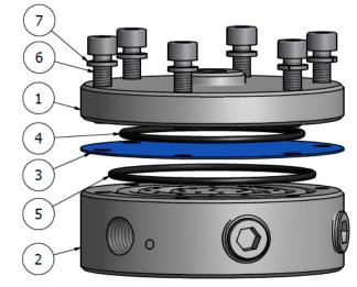
Figure A: Exploded View Standard Model
