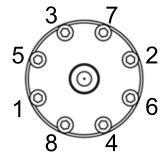
Figure B: Sample Torque Pattern
