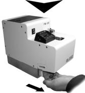
Return your hand to front with care not to drop the screws off your palm. The LCD panel LED goes out and the feeder restarts.
