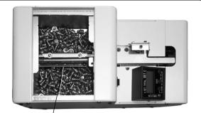
Do not allow screws hide the top surface of the rail groove. (The screws must be positioned about 2 to 3 mm lower than the top surface of the groove.)
