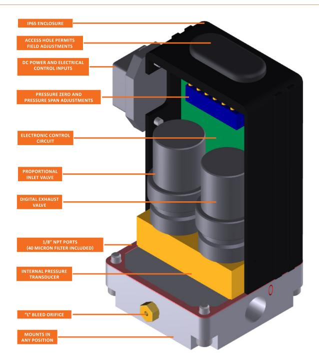
The Equilibar® QPV series electronic pressure regulator uses advanced technology circuitry to drive a true proportional response solenoid valve to provide improved resolution, near zero dead band, and longer solenoid valve life.
