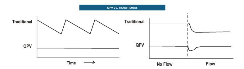
When flow or leakage is present in the system, traditional two valve I/P's bleed down and then actuate the inlet valve to compensate. This gives erratic pressure and flow. The QPV opens its inlet valve proportionally to match the system flow, resulting in steady pressure.
