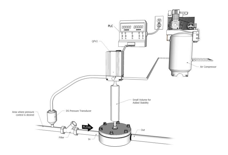
There are often applications where a user desires to control pressure in one part of an installation but needs to install the pressure regulator elsewhere. For example, having a filter, a long length of pipe, or some other obstruction before a back pressure regulator. As debris is collected in the filter the pressure drop across the filter changes, but the back pressure regulator is only capable of controlling the pressure between itself and the filter.
