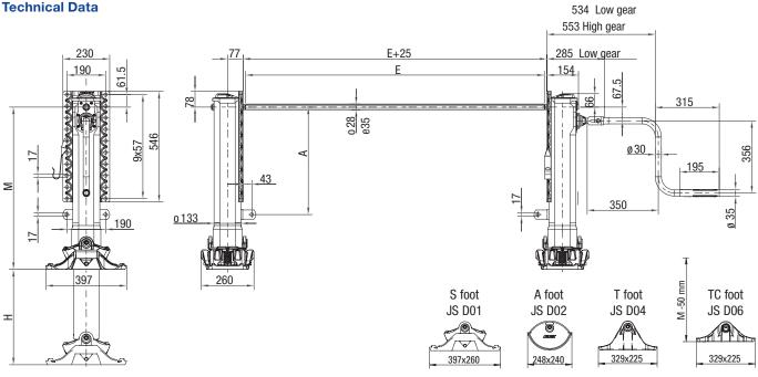
The drift for the S and A foot is  $\pm$  140 mm.
