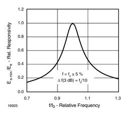
Fig. 5 - Frequency Dependence of Responsivity
