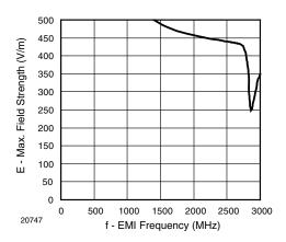
Fig. 7 - Sensitivity vs. Electric Field Disturbances
