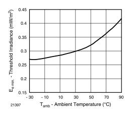
Fig. 8 - Sensitivity vs. Ambient Temperature
