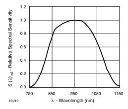
Fig. 9 - Relative Spectral Sensitivity vs. Wavelength
