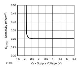
Fig. 11 - Sensitivity vs. Supply Voltage
