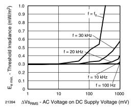
Fig. 6 - Sensitivity vs. Supply Voltage Disturbances
