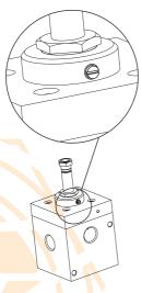
SM device installation on solenoid valve art. 07 .. 40
