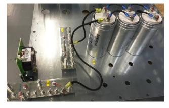
The EPCOS capacitors have been released for new built systems as well as for refurbishment of the existing Gutor UPS line XXW, based on the theoretical calculation of operational lifetime, the confirmation by the accelerated lifetime tests and the final overall UPS system test.
