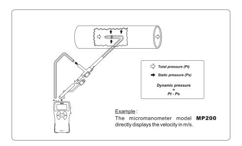
With the dynamic pressure in mm H<sub>2</sub>O or in Pa, we can calculate the air velocity in m/s, with the simplified BERNOULLI formula :
