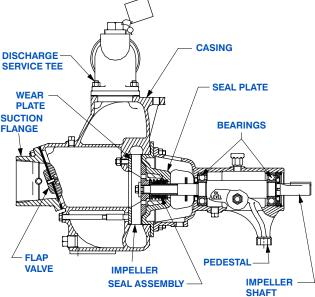
83A52-B SEAL DETAIL Type 31, Mechanical, Self-Lubricated. Silicon Carbide Rotating and Stationary Faces. Fluorocarbon Elastomers (DuPont Viton® or Equivalent). Stainless Steel 18-8 Cage and Spring. Maximum Temperature of Liquid Pumped 160°F (71°C).\*
