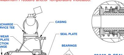
83A3-B SEAL DETAIL Type 2, Self-Lubricated. Mechanical. Carbon Rotating Face. Ceramic Stationary Face. Buna-N Elastomers. Stainless Steel 18-8 Cage and Spring. Maximum Temperature of Liquid Pumped, 160°F (71°C).\*
