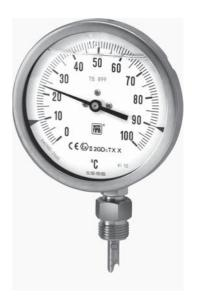
These instruments are designed for explosive atmospheres in food, processing, pharmaceutical, petrochemical industries and conventional and nuclear power plants. They are in conformity with the essential Health and Safety Requirements laid down in European Directive 2014/34/UE for Group II, Category 2G or 2GD equipment in the T1...T6 temperature classes. They are NOT suitable for ZONES 0 and 20.
