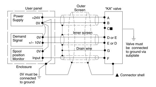
■ Spool position monitor voltage (pin F) will be referenced to the KA valve local ground. A "local ground" (pin C) is provided for optional use by differential input customer supplied electronics.
