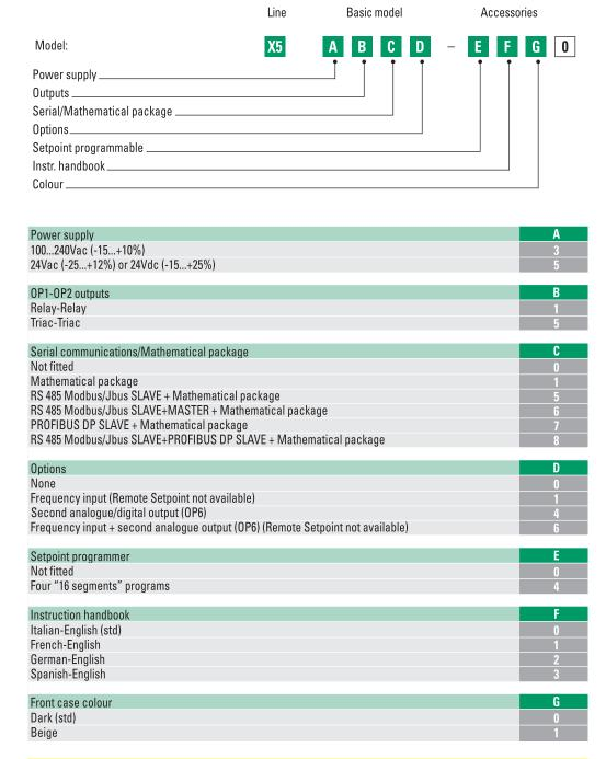
If not differently specified the controller will be supplied with standard version Model: X5 3100-0000
