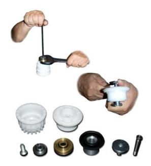
Unscrew the valve seat from the body (2), paying attention not to damage the sustain rims;
