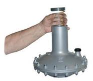
Remove the screws (47) that fix the low support cap (310) with the high support cap(340);
