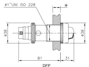
Threading 1" ISO 228 Lamp holder E14 Power ≤ 5 W Weight: 210 g
