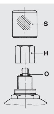
Gas valve for bladder accumulators
