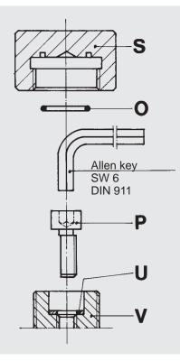
Gas valve for piston and diaphragm accumulators
